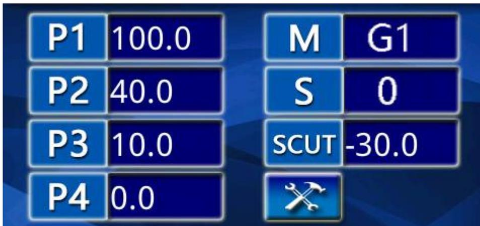
Note: The signal point setting value needs to meet the following requirements: P1>P2>P3>P4.
