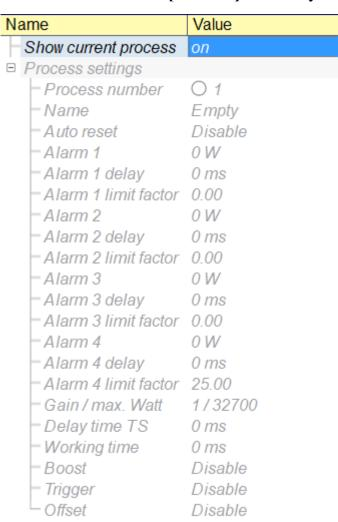
The alarm signal point is set based on the power value curve displayed by the software in the actual working state of the machine tool.
