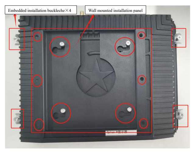
Embedded installation hole size: 274mm × 203mm
